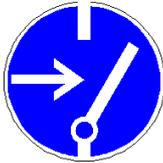
No part on which maintenance is performed can be under voltage. It is necessary to check with a two-pole measuring instrument that the disconnected parts are not under voltage, then connect them to ground and insulate the surrounding parts under voltage!
