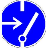
All parts maintained or repaired must be disconnected from the power supply. You must check that the disconnected parts are not under voltage by means of a bipolar measuring device, then connect them to the ground, and isolate neighbouring parts under voltage!
